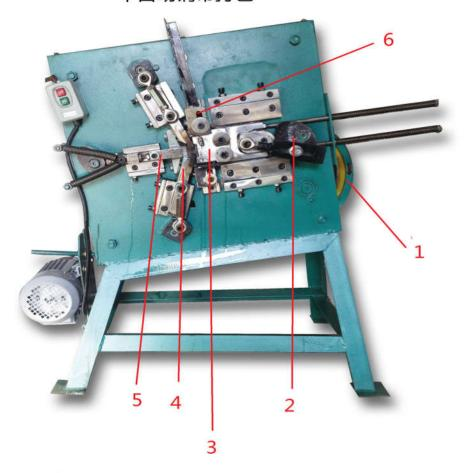
1.皮带轮 Pulley belt 2.偏心轮 Eccentric gear
